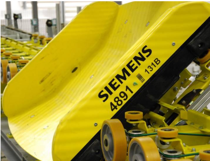
The tilt-tray conveyor uses a belt conveyor to move baggage items on to chutes that transfer them to the final station before they are loaded on to aircraft.
